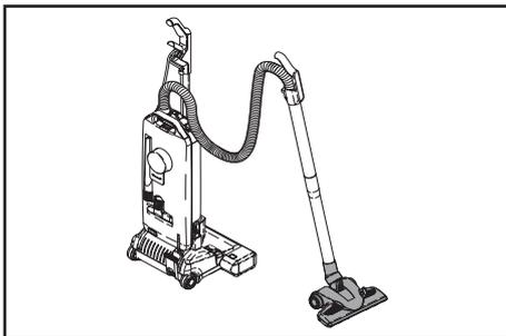
The hose(6) can be used on its own. For these purposes, please push the button(28) on the backside of the tube(7) and extracted the hose(6) out of the tube(7). After using put back the hose into the tube. The attachments(17,18) fit either to the end of the hose or the end of the tube.
